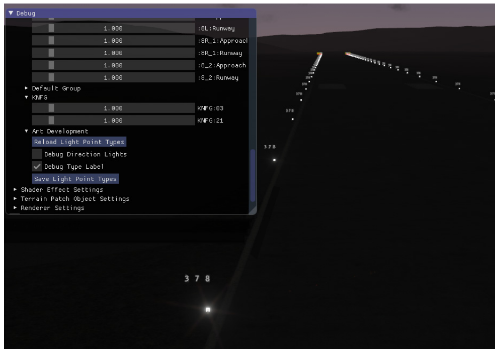
Figure 5-3. Lightpoint type labels
