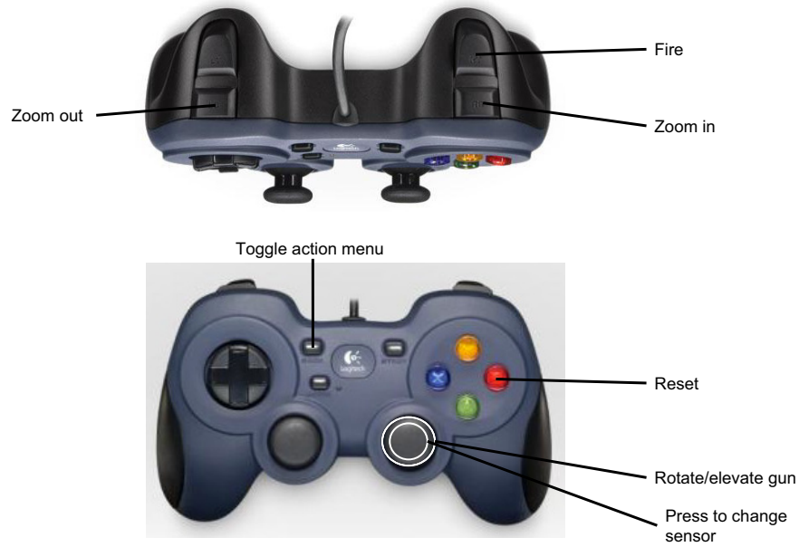
Figure 2-5. LAV gunner controls
