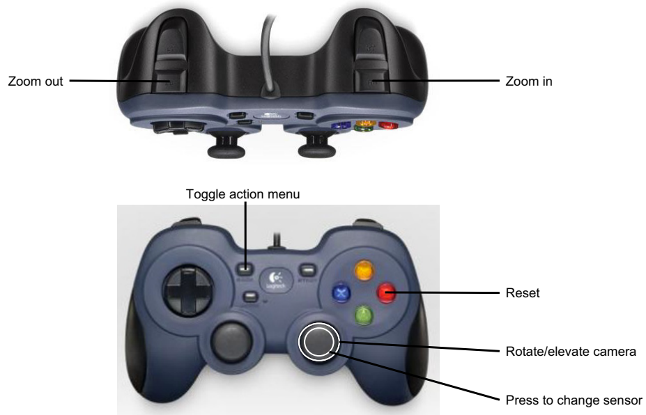
Figure 2-4. LAV commander controls
