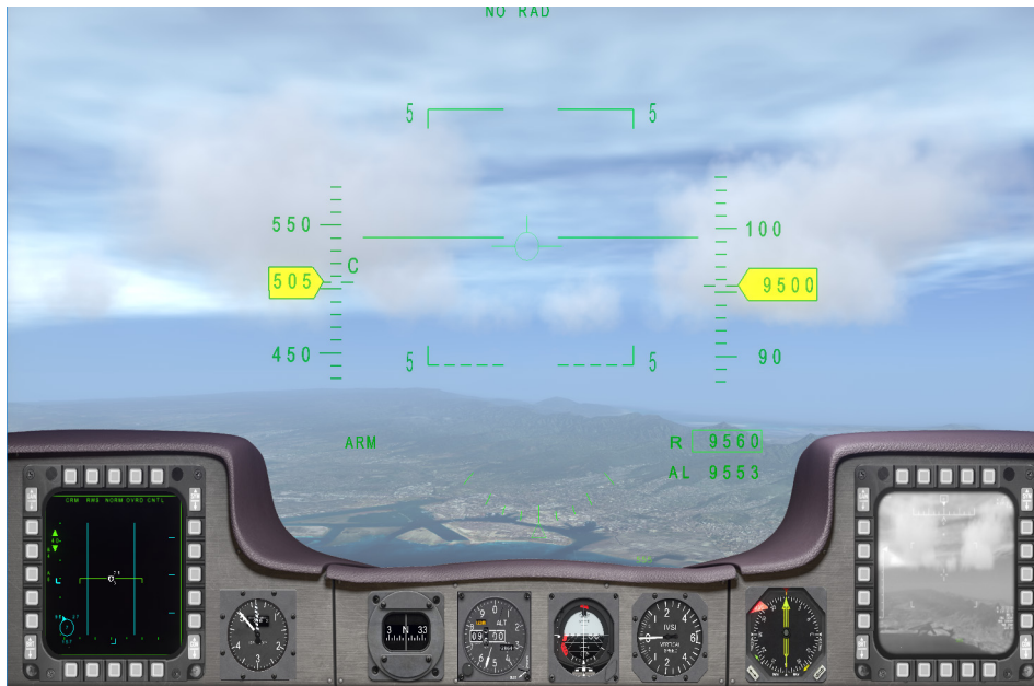
Figure 1-25. HUD and instrument panel (1 Screen Landscape display)
