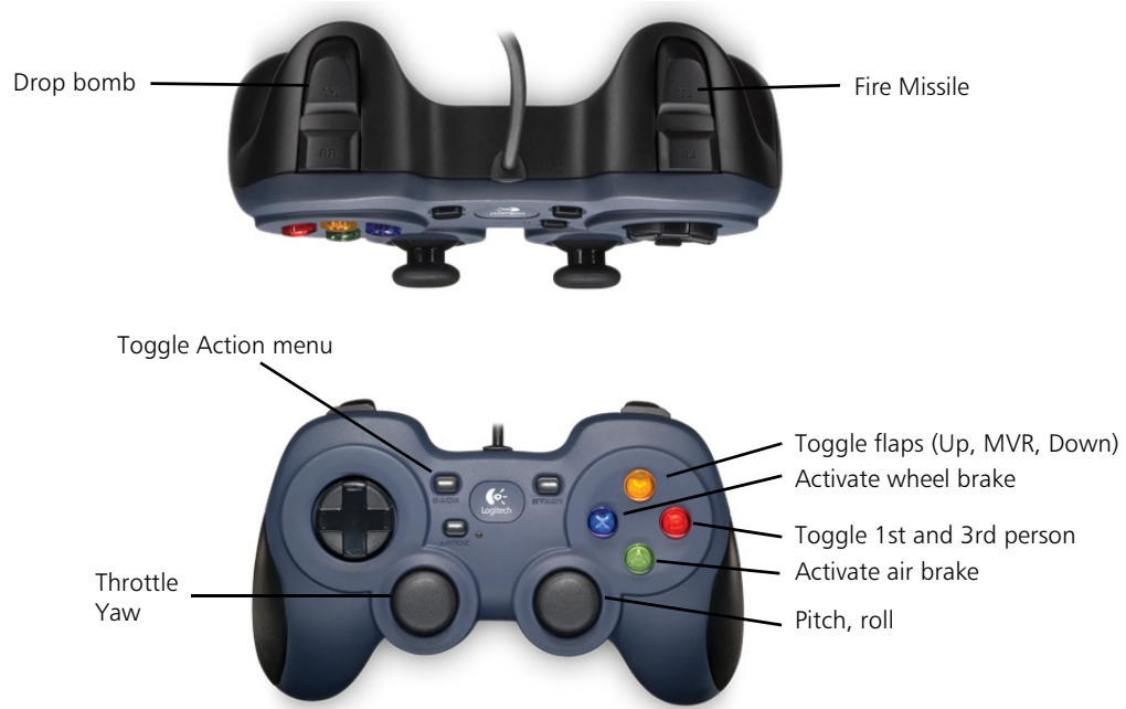
Figure 6-16. Fixed-wing flight controls
