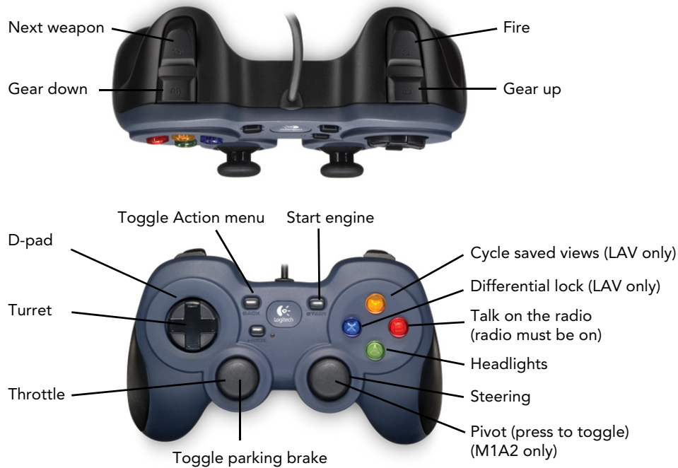
Figure 4-3. Driver controls for LAV and M1A2
