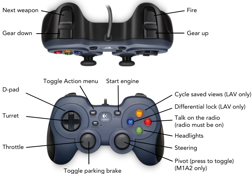
Figure 4-3. Driver controls for LAV and M1A2
