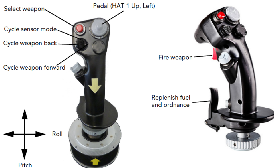
Figure 87. Thrustmaster HOTAS Warthog joystick mappings - rotary-wing
