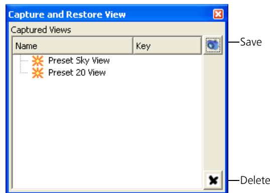
Figure 8-12. Capture and Restore View toolbar
