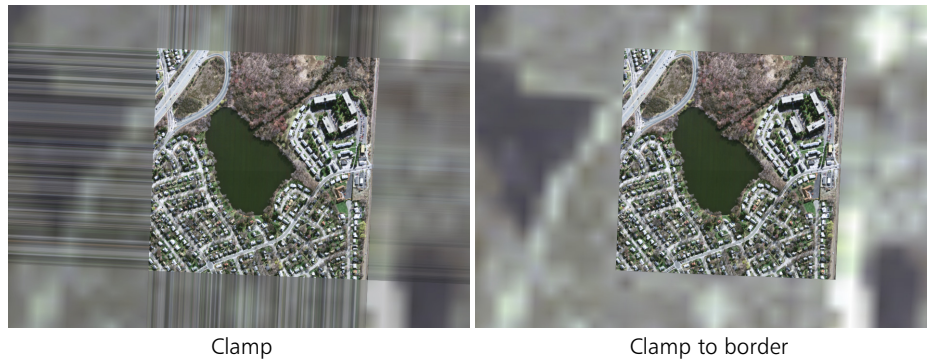
Figure 11-4. Raster image wrap effects (Clamp and Clamp to Border)
