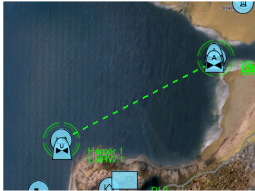
Figure 8-11. Radio communications line and squawk indicators
