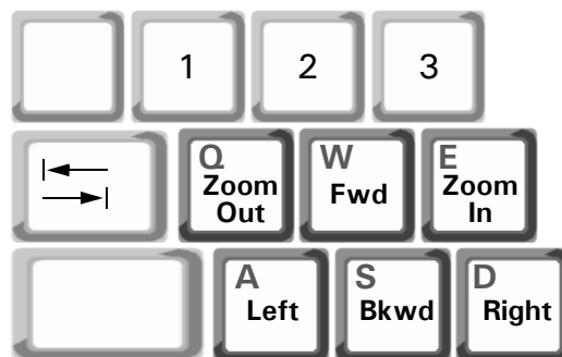
Figure 1-8. Primary movement keys, observer coordinates (2D)
