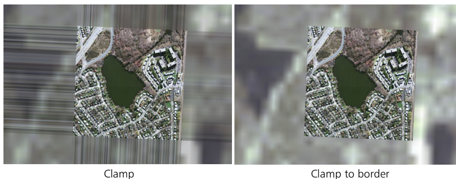
Figure 3-5. Raster image wrap effects (Clamp and Clamp to Border)
