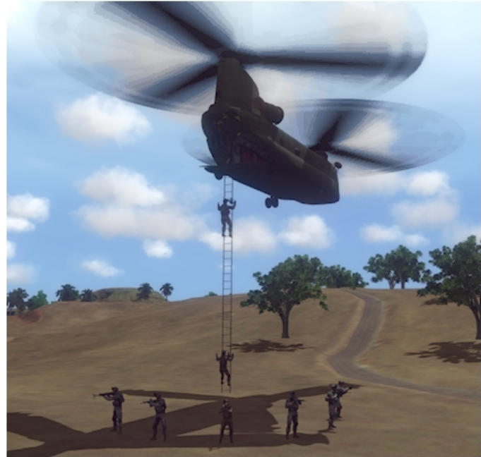
Figure 32. Ladder Insertion with Use Cargo Door and with Rope Ladder system positioned at rear of vehicle
