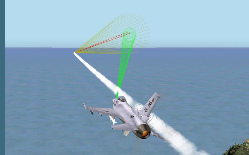
A/C radar illuminates target (green cone), missile radar locks on return echoes (brown cone)
